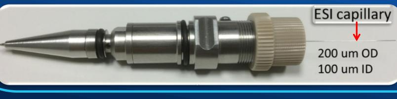
nis stainless steel capillary as been replaced with a old coated plastic version.
