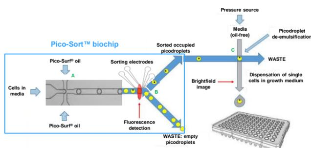
Figure 1: Schematic of the microfluidic process.
