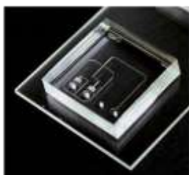
Figure 1: Pico-Gen™ biochip for picodroplet generation.
