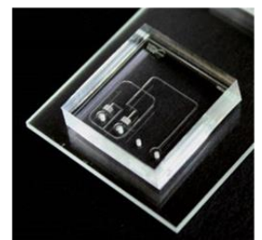
Figure 3: A Pico-Gen™ biochip for picodroplet generation.
